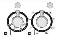
The Multi-function oven has two controls, a function selector and a temperature setting knob.
